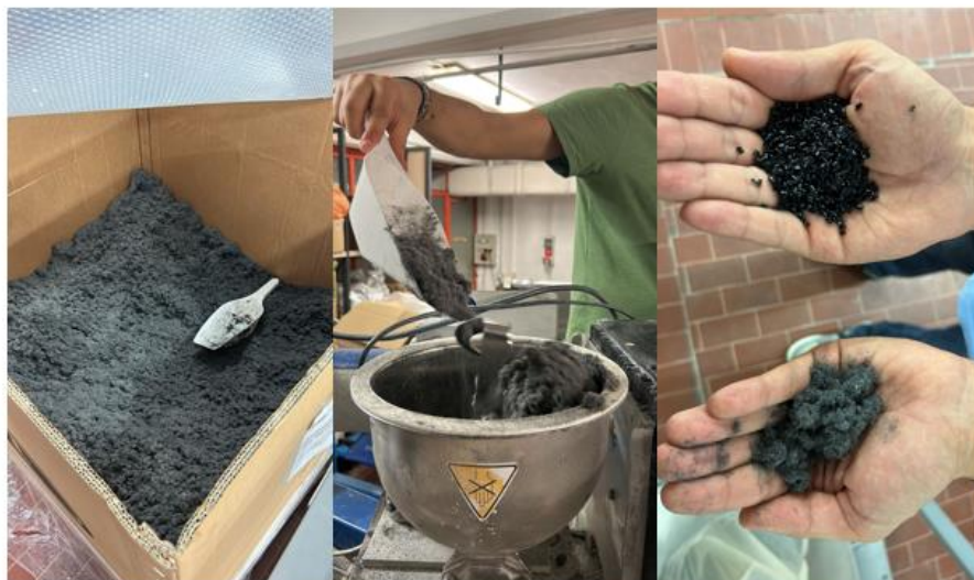
Safety belts powder from grinding
