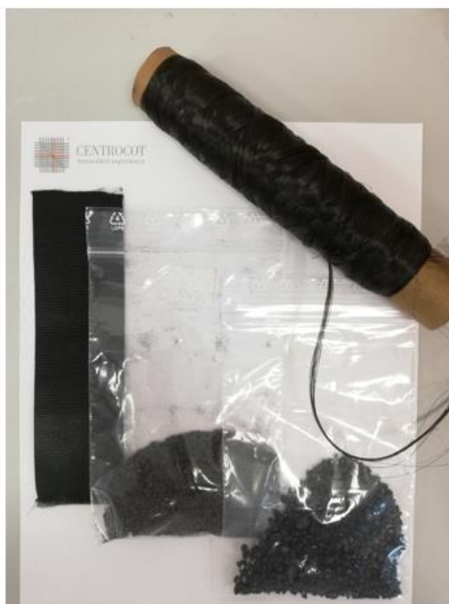
Safety belts → Powder → Pellets → Yarn
